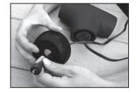
Hand-tighten the lonGen™ Probe collar into position.
